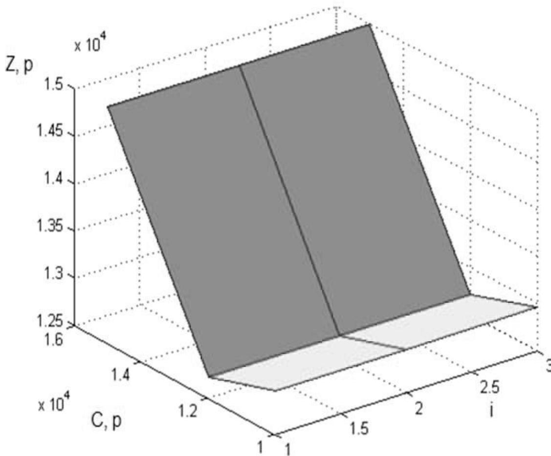
Fig. 2 Three-dimensional dependence of costs  $Z$  on the cost of static capacitors batteries and the number of its steps
