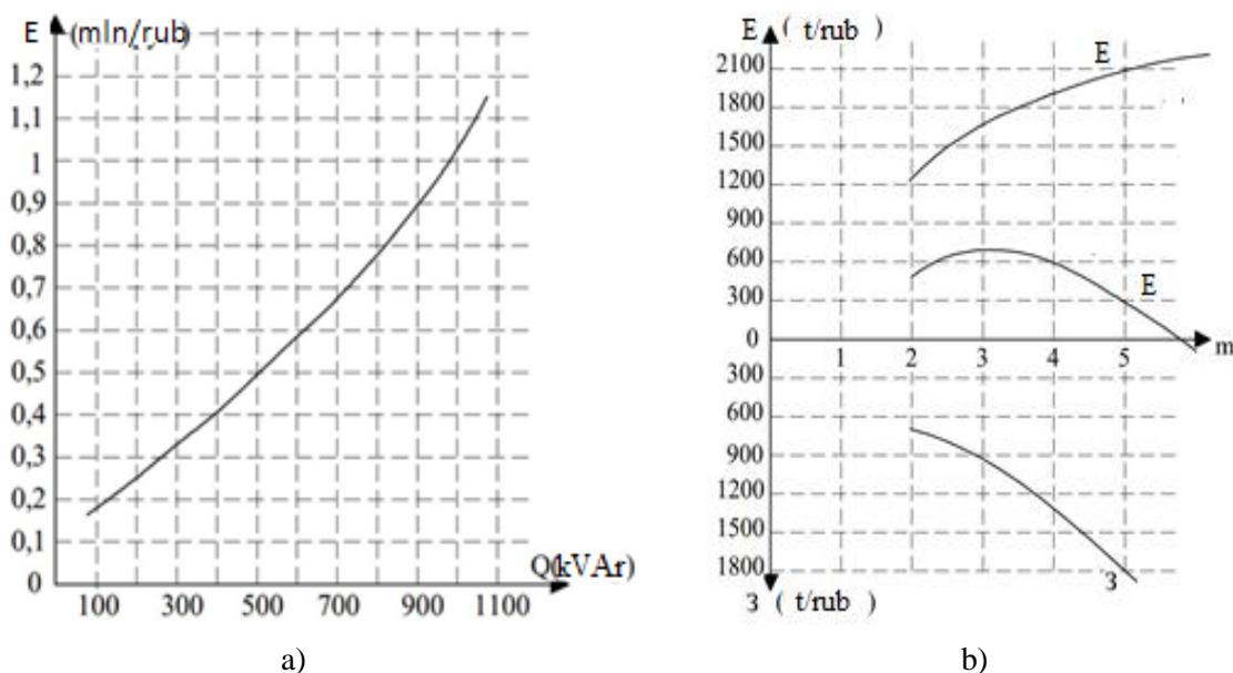
Fig.1. Functional dependences of price (a) and averaged efficiency (b) of high voltage PFC units use.
