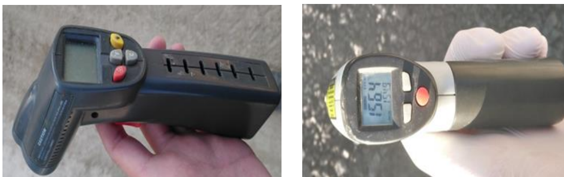
Figure 1. Remote thermometer for measuring asphalt temperature during installation
