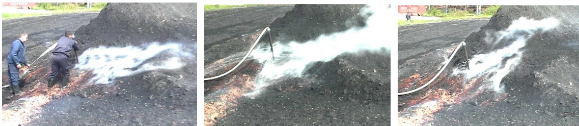
Slike 7, 8, 9. Faze gašenja požara – pobijanje mlaznice u dublji dio depoa Pictures 7, 8, 9. Phases of firefighting - the refutation of the nozzle in the deeper part of the depots
