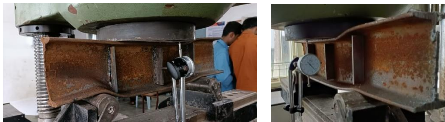
Figure 3. Beams at Failure
