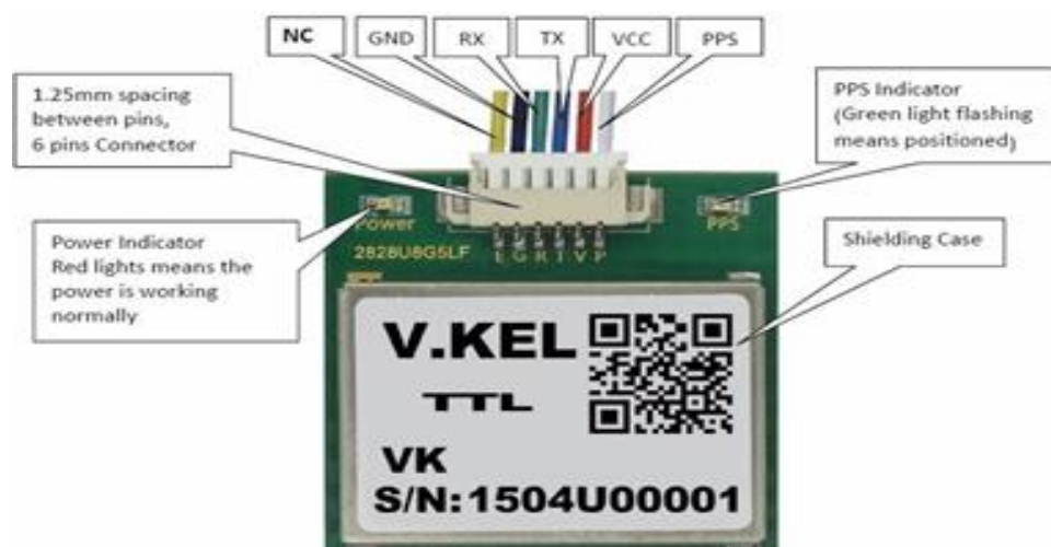
Figure 3. GPS U-blox (UBX-M8030-KT) module connected to Arduino [28]
