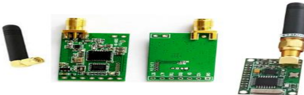
Figure 5. Transmitter/receiver 433-MHz RF LoRa and antennas
