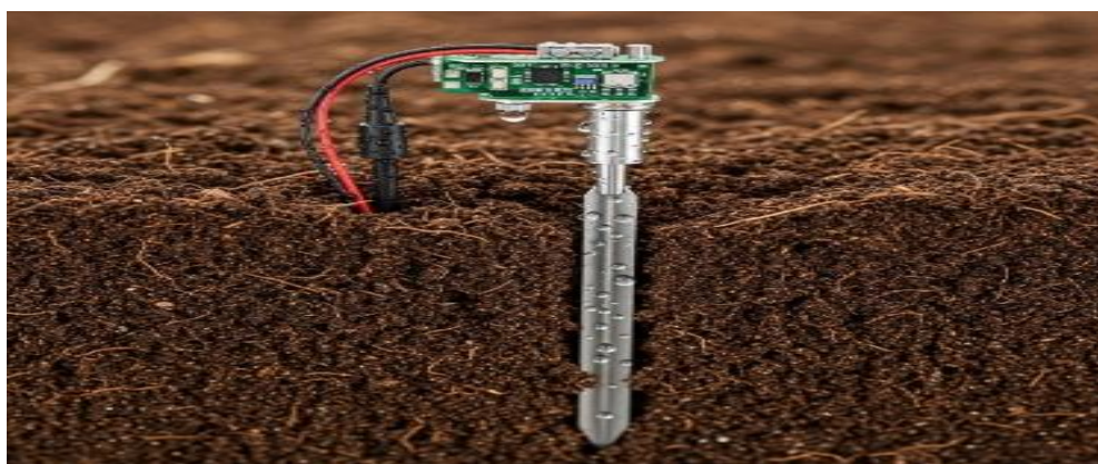
Figure 1. Soil moisture sensor and probe mechanism
