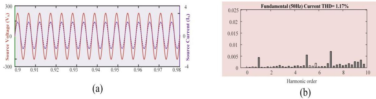
Figure 6. Simulation results illustrating the performance of the optimised converters operating with PIM control at  $V_s = 230V$ . (a) Representations of steady-state wave shapes detected at the source terminals (b) Harmonic spectrum investigation highlights the THDs
