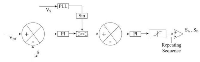
Figure 5. Closed-loop control architecture for the projected converters
