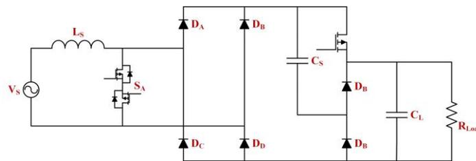
Figure 1. Architecture of the proposed SC-integrated power factor correction converter
