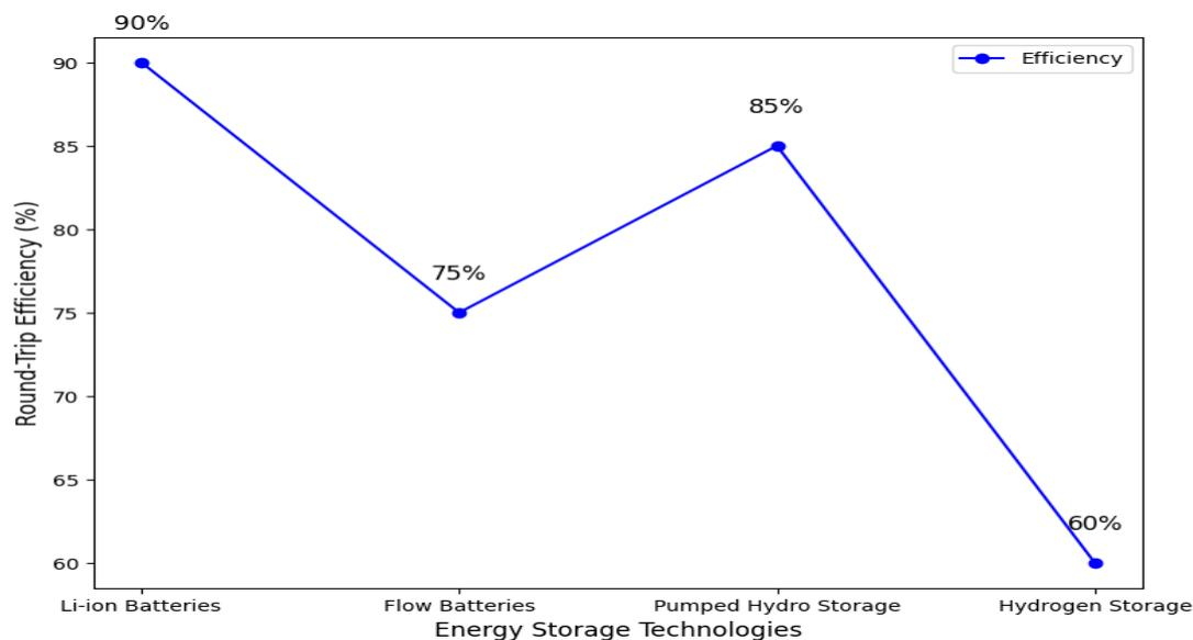
Figure 2. Round-trip efficiency of energy storage technologies
