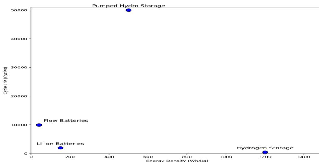
Figure 3. Energy density vs. cycle life for energy storage technologies
