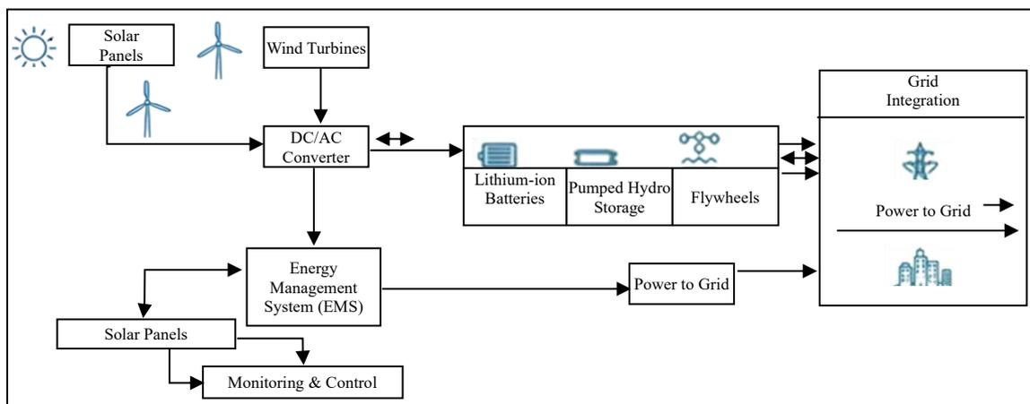
Figure 1. Architecture framework for renewable energy storage integration
