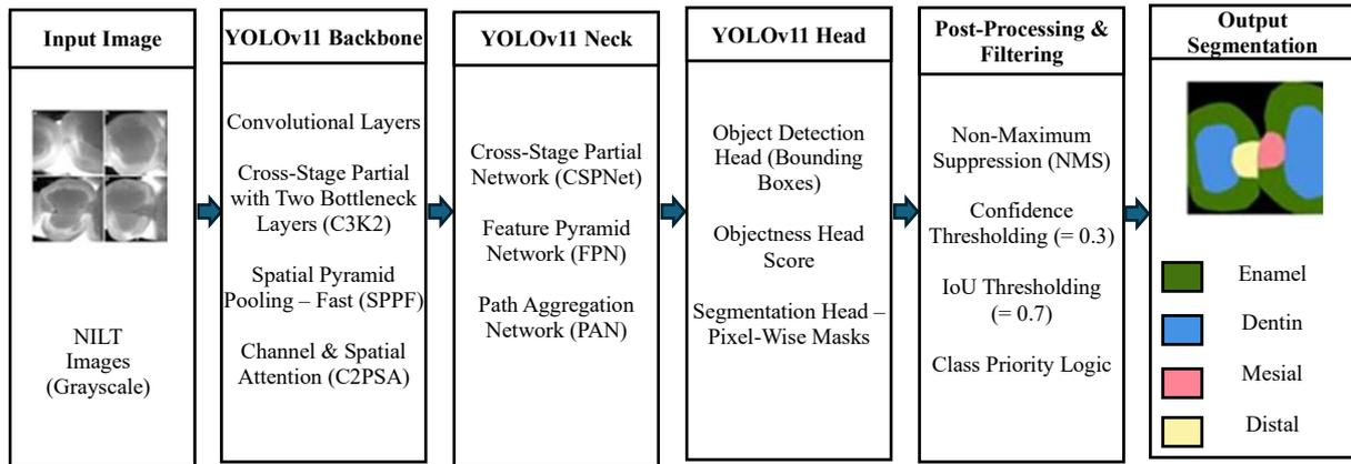
Figure 1. YOLOv11 Segmentation pipeline for proximal caries detection in near-infrared light transillumination (NILT) images
