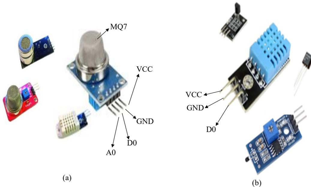
Figure 2. (a) Air quality sensor (b) temperature sensor
