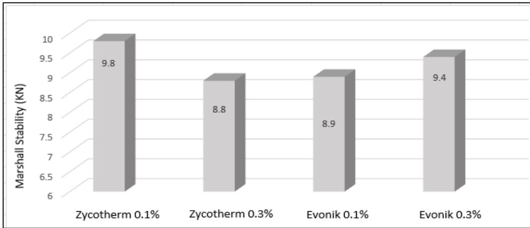
Figure 4. Marshall stability values of asphalt mixtures. fountain: [13]
