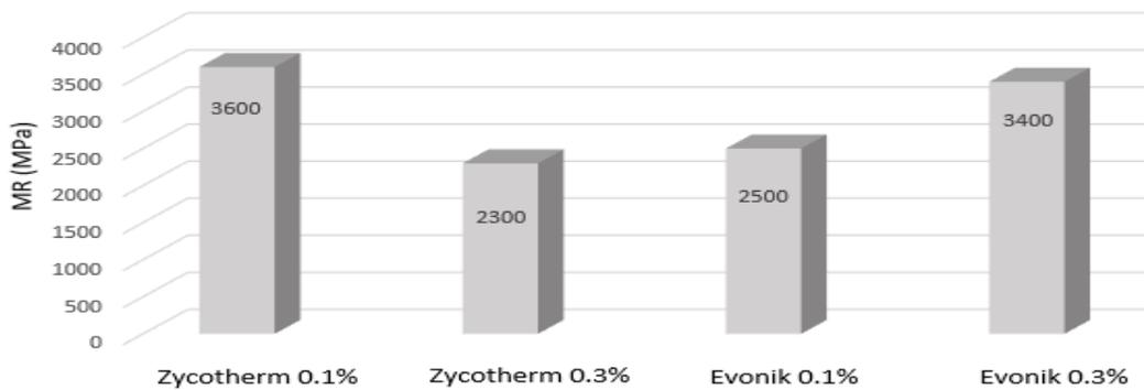
Figure 7. Resilient module test results. fountain: [13]
