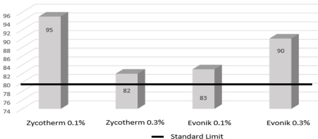
Figure 6. Tensile strength ratio values of modified asphalt mixtures. fountain: [13]
